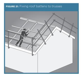
Roofing work involves several tasks that potentially expose persons to the risk of falls both through and from the edge of the roof structure. Physical edge protection must be provided for all roofing works, so far as is reasonably practicable.
