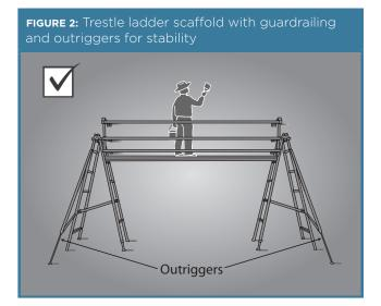
When adjusting the height of a brick layer's trestle scaffold, make sure that only the purpose-designed pins are used. Do not use nails or pieces of reinforcing bar.
