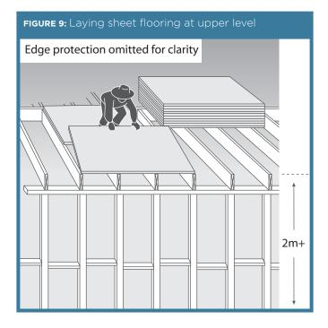
Safe access and egress must also be provided to the area where flooring is being laid. Access should be restricted to only those workers who are laying the flooring and erecting the wall frames.
