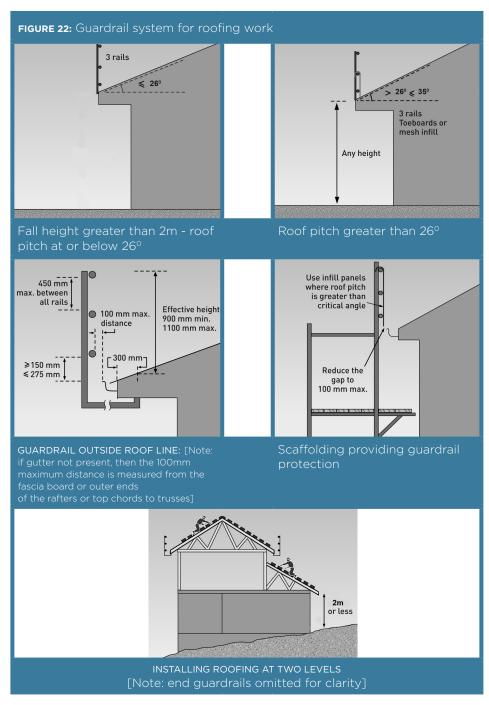
■ infill panels where the pitch of the roof exceeds 26 degrees.
